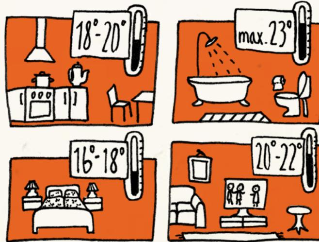
*Rooms must not all be equally warm. 18-20 degrees is sufficient in the kitchen, a maximum of 23 degrees in the bathroom, 20-22 degrees in the living room and 16-18 degrees in the bedrooms.*
